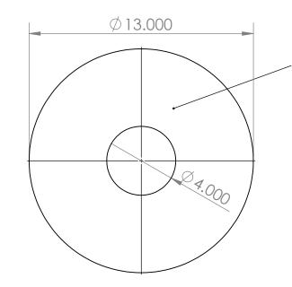
The dimensions of this flatented part are approximated to allow for the part to be drawn into the final shape (right) and to later be seamed with the stove body. These dimensions may need further refinement.
